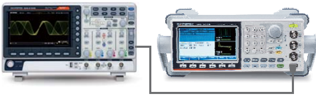
Direct Waveform Reconstruction from the DSO
