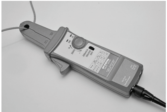
Figure 2. Connecting the GCP-300 current probe.
