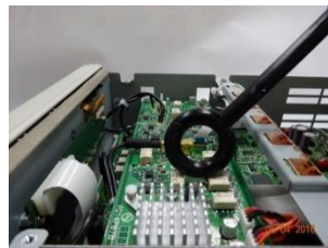
The measurement of conventional magnetic field probe
