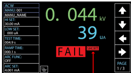
SHORT Status detected
