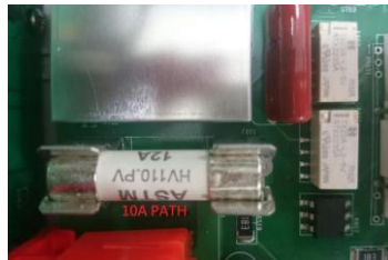
Internal 10A input current fuse
