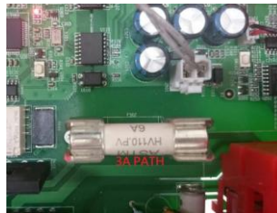
Internal 3A input current fuse
