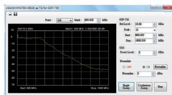
Test Result of Low Pass Filter with PrimaryRF Software
