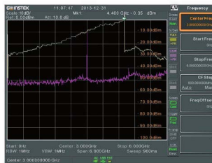
Test Result of Simultaneous Power Sweep and Frequency Sweep
