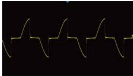
TrailingEdge phase dimming
