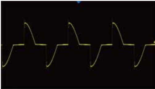
LeadingEdge phase dimming
